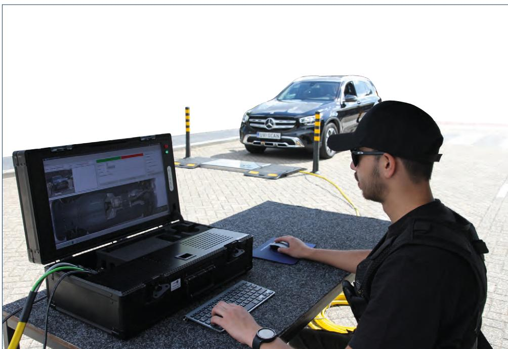
Install the guiding poles to make sure that the vehicles drive correctly over the Scanning Unit, with the wheels on either side.
