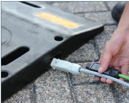
Place the 4 UVIScan rubber mats on the frame. Take the yellow cable and insert the 2 connectors for the Scanner carefully through the rubber mat ducting.
